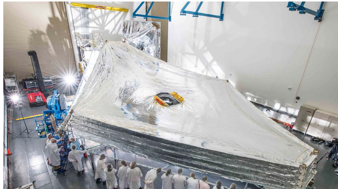
The sunshield of NASA's James Webb Space Telescope is the size of a tennis court and constructed of five individual layers of Kapton, a polyimide film that can withstand the harshest of conditions. Deployed sunshield models undergo testing at our Space Park facility in Redondo Beach, California.
